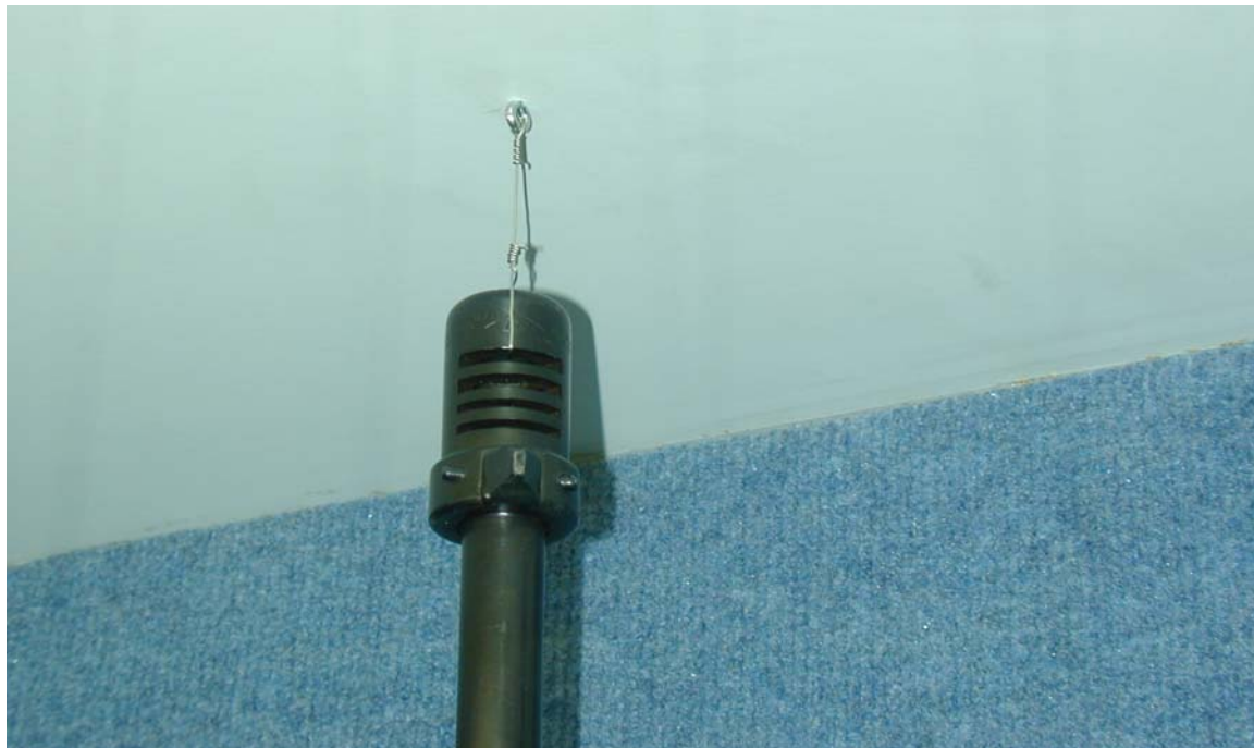
Close up of the bolt and wire suspending the TSMG from the ceiling of the display cabinet.
